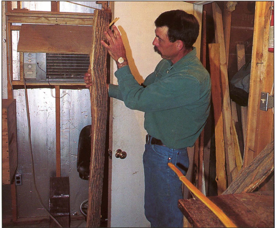
Selecting wood is the first step. Dowell uses Osage orange, which is tough and durable. The wood must first be dried to less than 10 percent moisture content.
